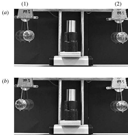
Figure 1. Multiple-exposure images illustrate the anti-phase attractor of a large mass ratio ( $\mu = 0.0063$ ) system of two pendulums mounted on a common translating beam. (a) The system is started with equal amplitude, in-phase oscillation of the left (1) and the right (2) pendulums. In the presence of weak coupling through lateral motion of the mounting cart, the in-phase state is unstable and, after a sufficient time, the system oscillates stably in anti-phase final state (b).
