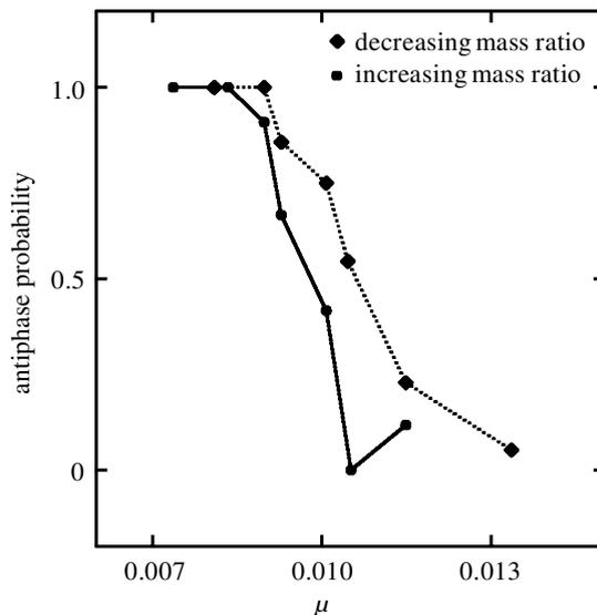
Figure 3. Probability of observing stable anti-phase oscillations as a function of mass ratio  $\mu$  for the clock system that begins at rest with both pendulums having in-phase angular displacements of equal amplitude. In this range of  $\mu$  only two asymptotic states are observed: anti-phase oscillation and beating death.
