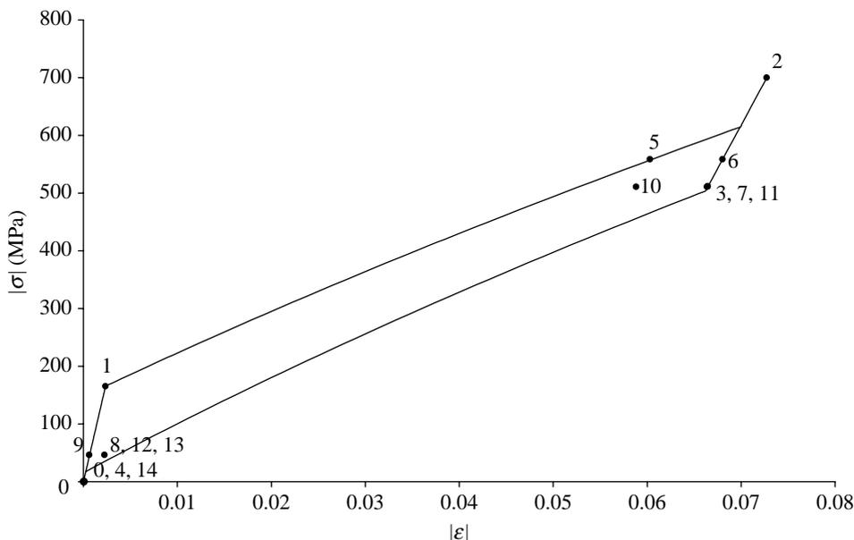
Figure 2. Stress–strain curve of the SMA under quasi-static loading/unloading.
