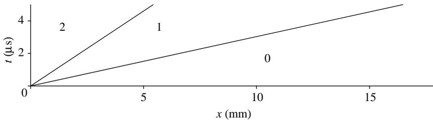
Figure 3. Shock waves and the regions of the piecewise constant solution during loading.
