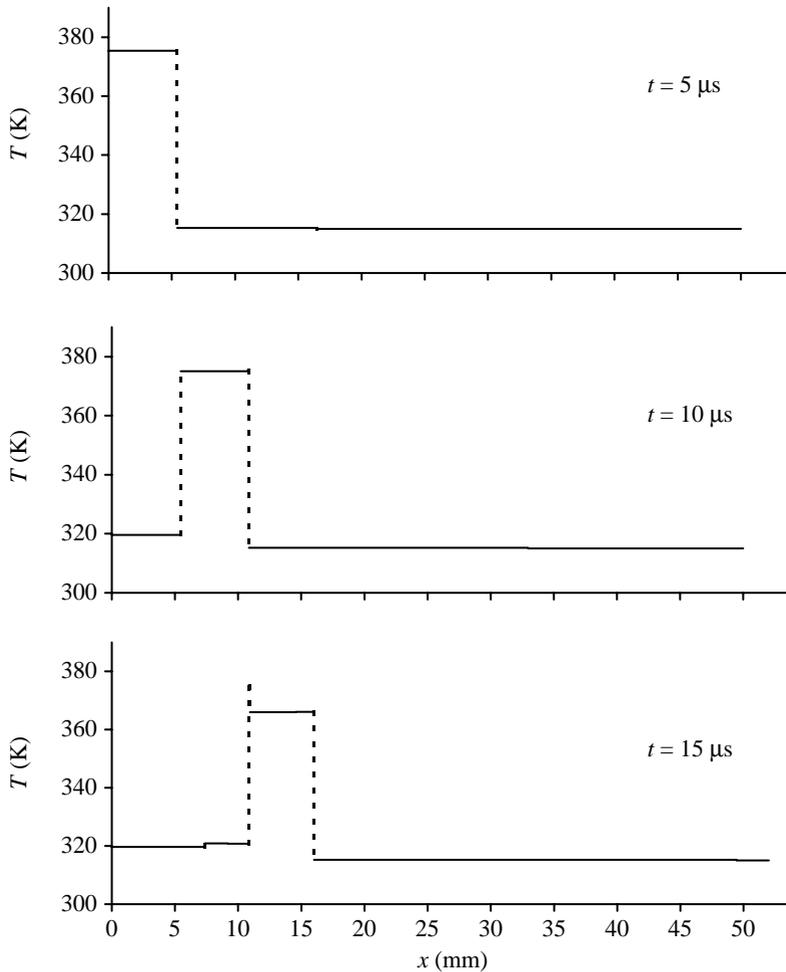
Figure 8. Temperature profiles at various times.
