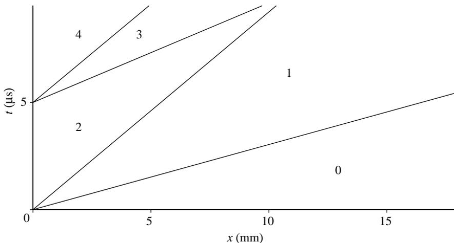
Figure 4. Shock waves and the regions of the piecewise constant solution during loading and initial stage of unloading.
