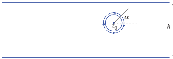
Figure 1. Circular treadmilling swimmer, of the type proposed in [7], centred at z_0(t) at orientation \alpha(t) in a channel of width h . The radius of the swimmer is \epsilon \ll 1 . Its evolution equations, correct to \mathcal{O}(\epsilon^3) , can be determined from the results in [4] using the transform results of §§3 and 4. (Online version in colour.)
