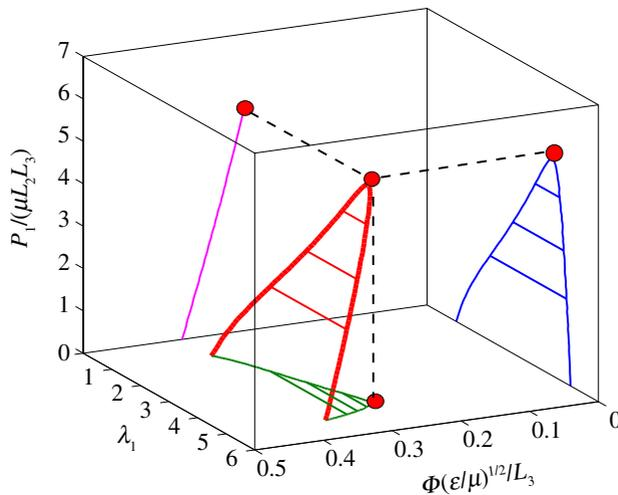
Figure 11. A three-dimensional representation of the electromechanical phase diagram for a dielectric elastomer membrane. (Online version in colour.)
