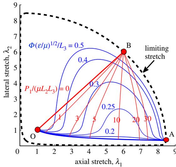
Figure 2. Curves of constant voltage and curves of constant axial force on the  $(\lambda_1, \lambda_2)$  plane for a dielectric elastomer membrane. The dashed curve is the boundary set by equation (2.14) for the limiting stretch of the elastomer ( $J_{lim} = 69$ ). (Online version in colour.)
