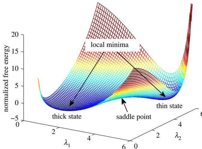
Figure 4. Normalized free energy as a function of the stretches for a dielectric elastomer under a uniaxial force  $P_1/(\mu L_2 L_3) = 1$  and a voltage  $\Phi/(L_3 \sqrt{\mu/\varepsilon}) = 0.337$ , showing two local minima and one saddle point. (Online version in colour.)
