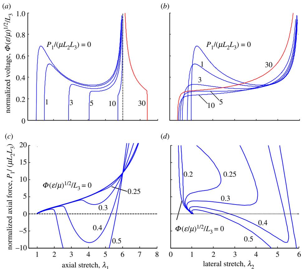
Figure 3. Stretches of a dielectric elastomer membrane caused by uniaxial force and voltage as predicted by the homogeneous solution. For constant values of the force: (a)  $\Phi - \lambda_1$  and (b)  $\Phi - \lambda_2$  curves. For constant values of the voltage: (c)  $P_1 - \lambda_1$  and (d)  $P_1 - \lambda_2$  curves. (Online version in colour.)
