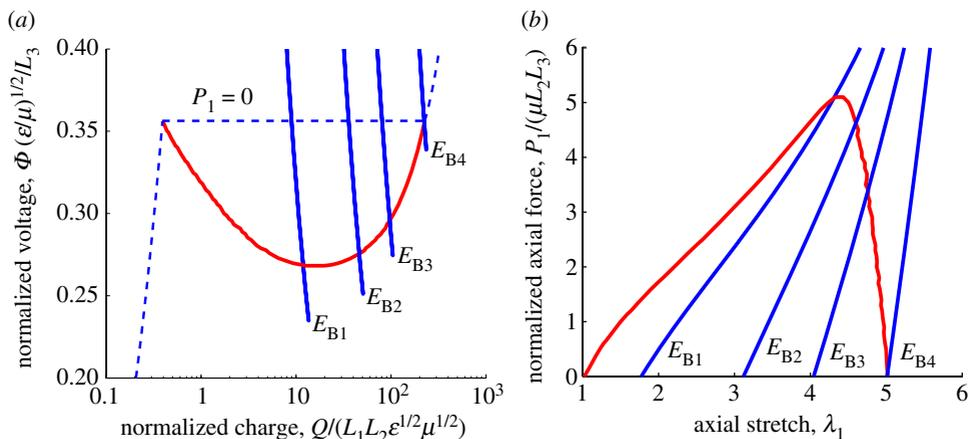
Figure 15. Electrical breakdown limits in (a) voltage–charge and (b) force–stretch diagrams, for  $E_B\sqrt{\epsilon/\mu} = 1.785$  ( $E_{B1}$ ), 3.570 ( $E_{B2}$ ), 5.355 ( $E_{B3}$ ) and 8.925 ( $E_{B4}$ ). The red curves are the electromechanical phase-transition lines ( $J_{\text{lim}} = 69$ ). (Online version in colour.)
