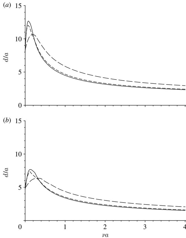
Figure 4. Bounds given by equations (7.7) and (7.11) for (a) two circles and (b) two ellipses with  $d/a=0.08$ , all submerged to a depth  $d$ :  $s=0$  (solid curve),  $s=0.2$  (short dashed curve) and  $s=1$  (long dashed curve). The uniqueness domain is located above the curves.
