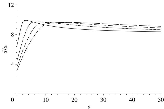
Figure 5. Bounds given by equations (7.7) and (7.11) for two circles submerged to a depth  $d$ :  $\nu a=0.5$  (solid curve),  $\nu a=1$  (short dashed curve),  $\nu a=1.5$  (medium dashed curve) and  $\nu a=2$  (long dashed curve). The uniqueness domain is located above the curves.
